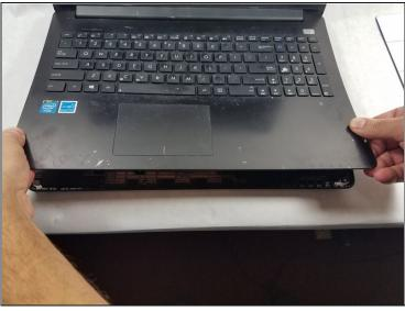
• Use the Plastic Opening Tool to pry the keyboard assembly away from the rest of the laptop.
