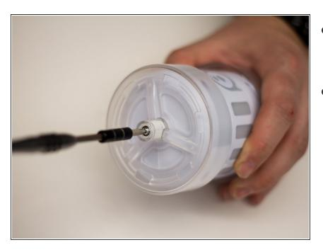
Loosen and remove the 10mm screw on each side of the device using a JIS 1 screwdriver tip.
