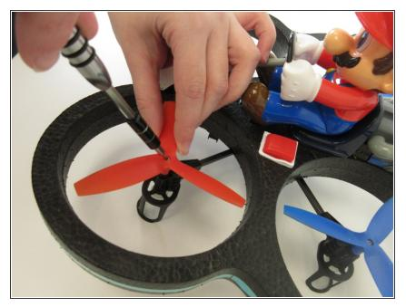
Using the JIS #00 screwdriver, hold the rotor blade still and unscrew the 4.762mm screw in the center of the blade.
