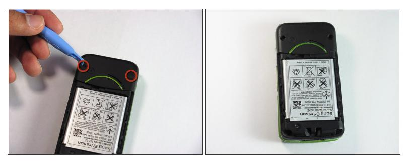
• Remove the two rubber casings for the top two screws with a plastic opening tool.
