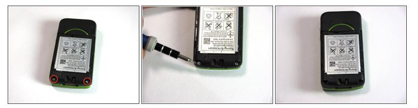
• Unscrew the bottom two 5.4mm screws with a Torx T6 screwdriver.
