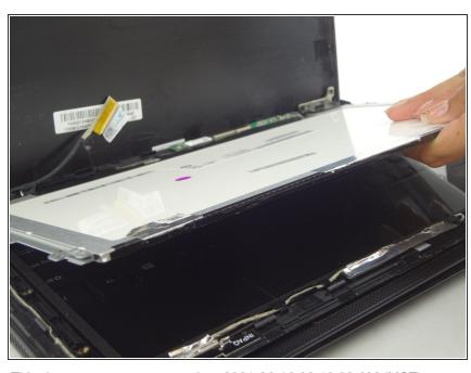
Lift the LCD screen to remove it from the device.
