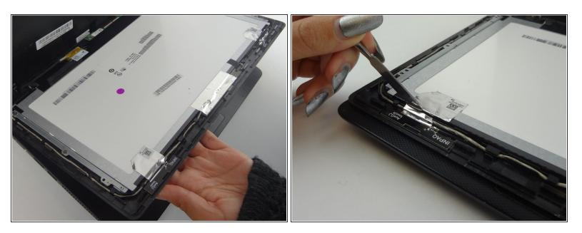
Slice the silver foil tape with a spudger by applying pressure between the frame and the back of the screen case.
