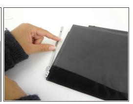
Remove the four silver 2.7 mm screws to separate the LCD screen from the two screen brackets.
