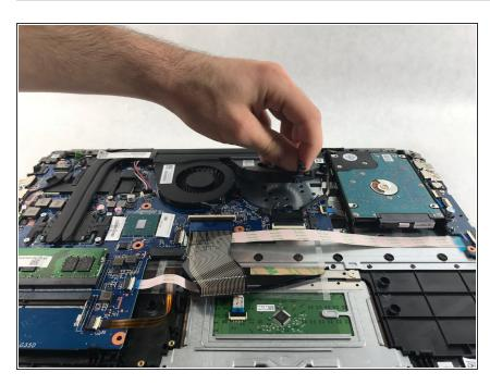
The fans can now be removed from the device.
