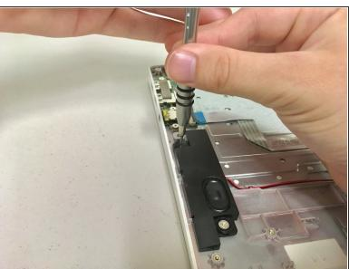
Unscrew the four 4mm Phillips screws.
