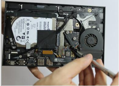
Remove the five screws using T6 Torx screwdriver.
