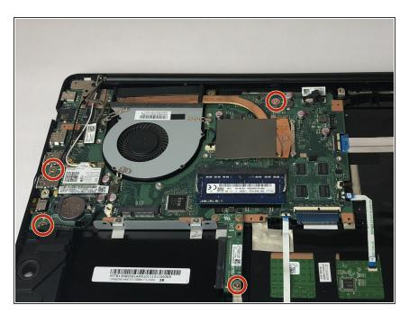
Remove the four 5 mm Phillips #1 screws around the perimeter of the motherboard.
