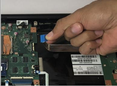
Remove the four ribbons connected to the motherboard.
