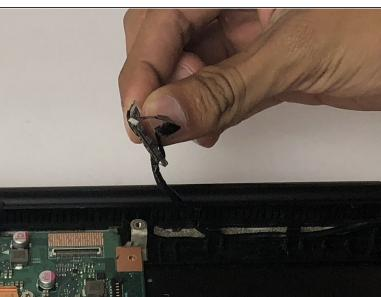
Disconnect the five wires attached to the motherboard by pulling gently. There are three thin wires in the upper left corner.
