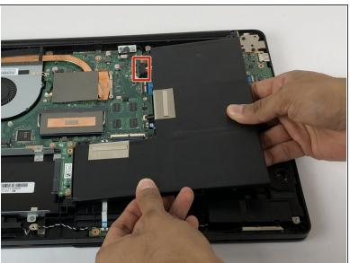
Using a plastic opening tool, lift the battery straight upward to remove it.
