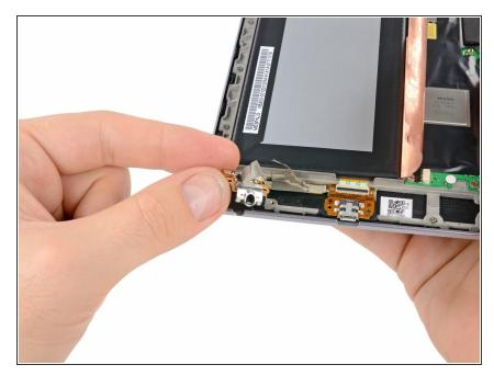
Without stressing the cable, and minding any tape that may still be holding the cable in place, gently lift the headphone jack up off its placement pins.
