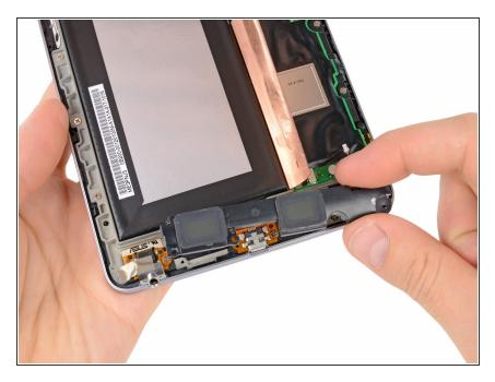
Lift and remove the speaker assembly out of the Nexus 7.
