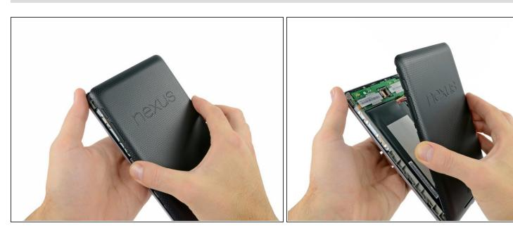
Gently lift and remove the rear panel up off the front panel assembly.
