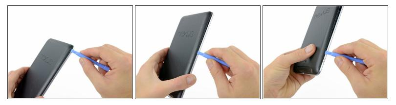
Pry up the rear panel along the left edge using the method described in previous steps.
