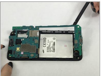
Carefully use the spudger to pry the motherboard out of the plastic tabs.
