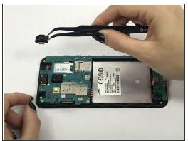
Remove connector tab with spudger then carefully remove headphone jack with tweezers.
