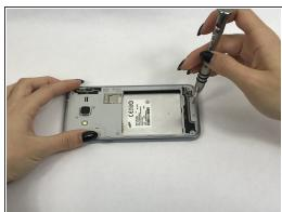
Remove the ten 2.0 mm screws with the Phillips #J000 screwdriver.
