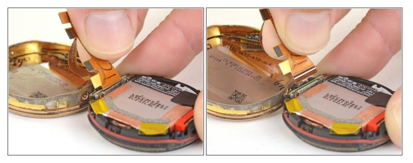
• Lift the display cable straight out of its connector on the motherboard.
