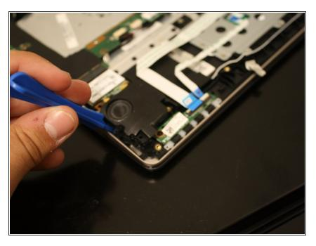
Use a long plastic pry tool to remove the speaker from the computer.
