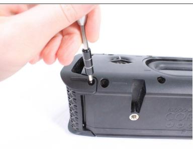
Remove the 8 screws (4 on each side) that hold the covers that conceal the bass speakers.
