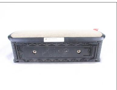
Using your hand, unscrew the large screws underneath the speaker.
