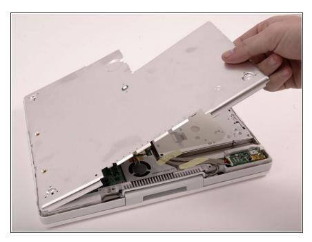
• Lift the bottom shield off.
