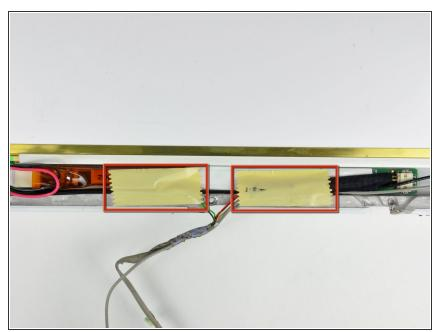
Remove the two pieces of tape covering the inverter/AirPort cables along the lower edge of the display.
