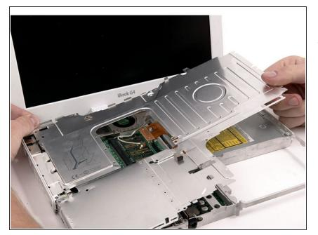
Lift the top shield up from the right side, minding the upper left corner, which may catch on the metal framework.
