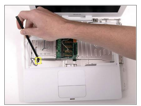
Lift the upper case off completely and disconnect the multicolored speaker cable from the logic board. As before, make sure you're pulling only on the connector and not on the socket.
