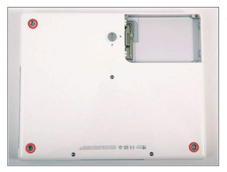
• Remove the three newly-revealed Phillips screws.
