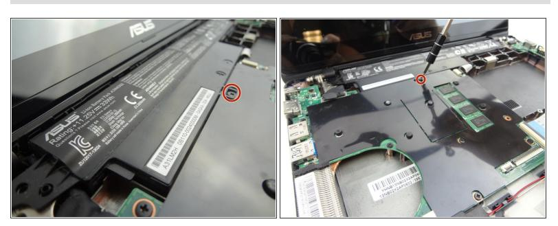
Use a Phillips #00 screwdriver to remove the black 4.7mm screw holding the battery in place.
