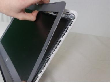
Gently pry around the edges of the display using a spudger to remove the bezel that borders the screen.
