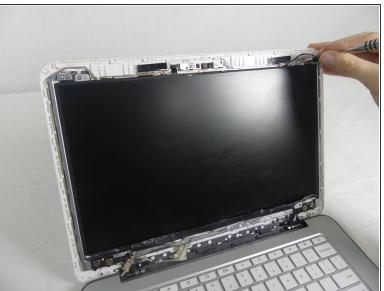
Once the bezel has been removed, remove the four 5mm screws at the corners of the screen using a PH00 screwdriver.
