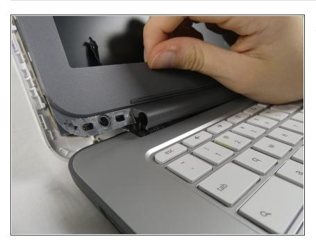
Once glue is separated, pop out the front cover by pulling upwards on the hinge.
