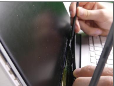
Remove glued plastic at the bottom of the cover.
