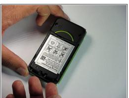
• There are eight snap hooks located around the outer case. Carefully snap these to remove the outer case.
