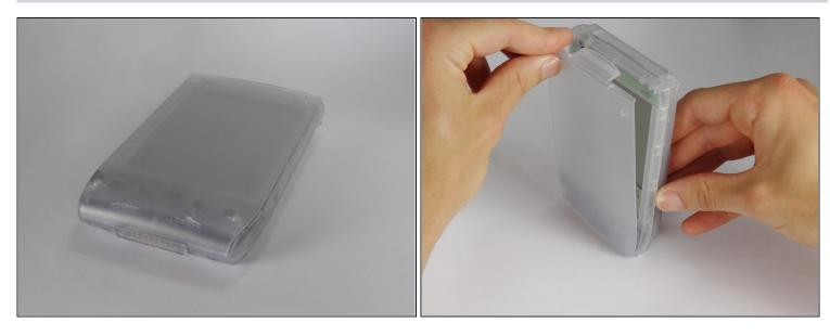
• Remove the outer screen cover by releasing the top clip from the main body of the device.
