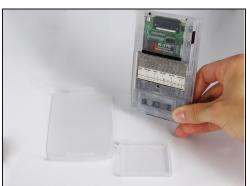
• Slide the memory cartridge cover up and off the device.
