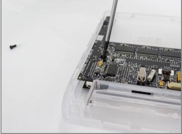
• Unscrew the two 2.94mm Phillips #00 screws that hold the motherboard in place.
