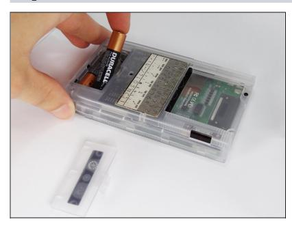
• Remove the batteries from the device.
