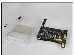
• Use the spudger to lift the motherboard from the case.
