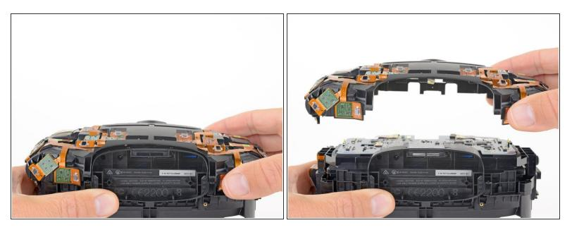
Lift the sensor array away from the headset to remove it.
