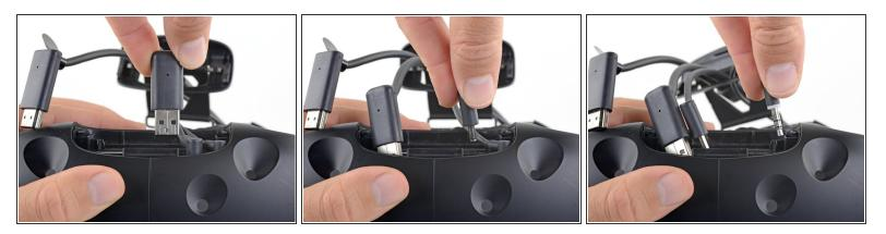
• Repeat the lifting and unplugging process with the remaining USB, power, and audio cables.
