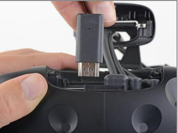
• Lift the HDMI cable straight up to unplug it from the headset.
