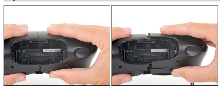
• Grasp the right half the outer shell and pull it to the right and toward the front of the headset in a twisting motion until you feel the clips on the front of the cover release.
