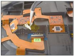
• Use <u>tweezers</u> to remove the clear tape over all four of the sensor array cable connectors.
