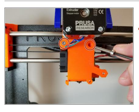
Remove the 2 X M3 Bolts from the Extruder Plate.
