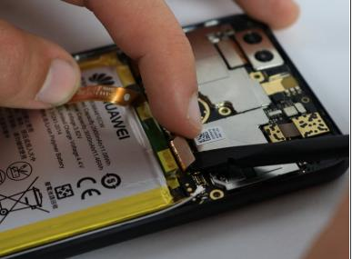
Using a spudger, gently pry up the small connection that holds the motherboard in place.
