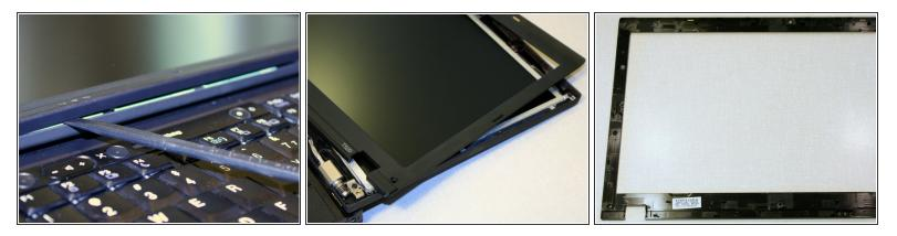
• Starting from the bottom of the screen, release the plastic clips holding the bezel by pushing horizontally inward and prying upward with a spudger.
