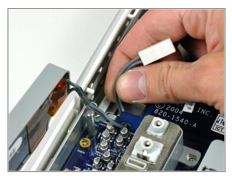
De-route the inverter cable connector from the channel in the logic board.
