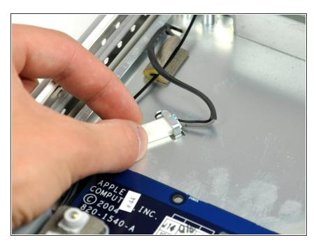
Slide the inverter-to-display cable connector from under the metal clip on the midplane.
