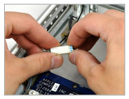
Disconnect the inverter-to-display cable connector by pulling it straight away from its socket.
