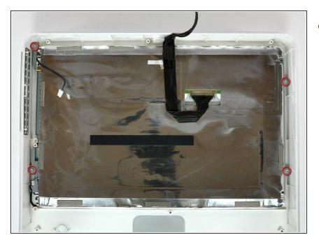
Remove the four T10 Torx screws securing the display to the front bezel.
