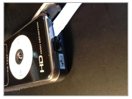
Now carefully using a spudger or case opening tool, carefully rise the front bezel from the back casing by working around the device.
