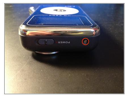
On the top side there is a screw (circled) that is under a little black dot. Peel that dot off with a knife or pointed spudger.
