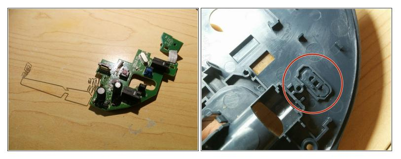
Carefully remove PCB. Take care not to bend battery connector
