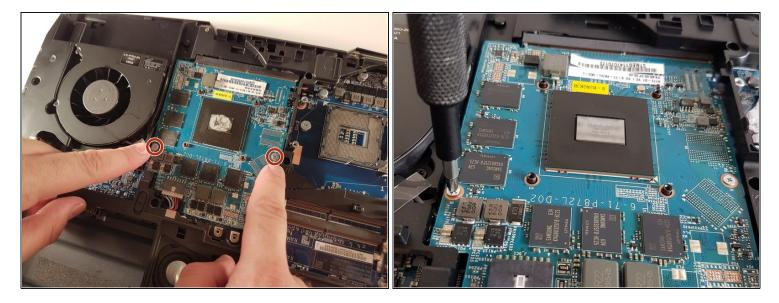
• Unscrew the two screws circled in red
