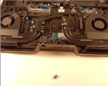
Unscrew the two screws circled in red
