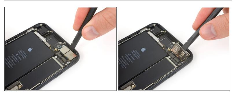
• Use the flat end of a spudger to pry up the rear-facing camera assembly from the top edge of the iPhone.
