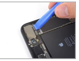
Use an iFixit opening tool or a fingernail to disconnect the two camera cable connectors by prying them straight up from their sockets.
