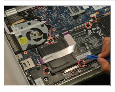
Remove the four Phillips M2.5x4.4 screws using the Phillips 00 located along the perimeter of the battery.
