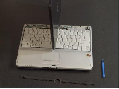
• There are four clip points at the bezel's rear, release each one and remove the bezel.
