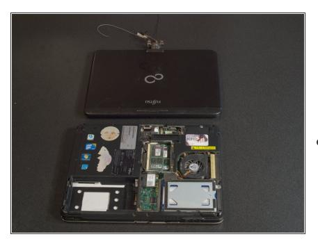
The display is now free. Carefully feed the delicate cables and connectors through the hole on the underside of the machine. Lift the hinge out of the laptop body. Be careful not to catch the cables near the hinge on the upper surface. These cables can be removed if you do not want to deal with working around them.
