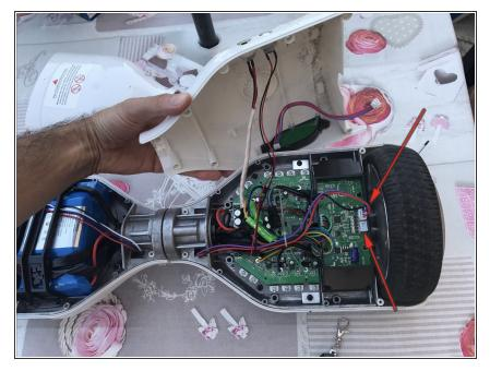
• Unhook the lighting and indicator light wires to remove the cover.
