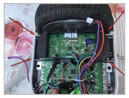
• Remove the 4 screws that hold the circuit board support.
