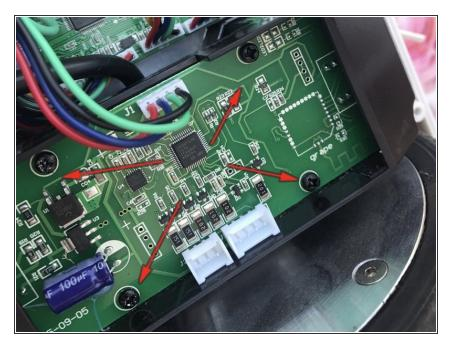
• Remove the 4 screws that secure the board to the support.
