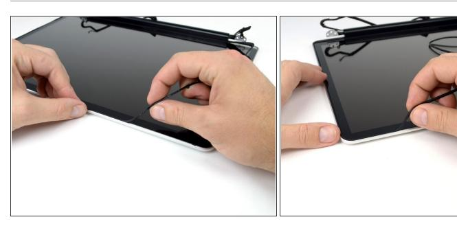
Continue pulling the display gasket off the display assembly across the top edge.
