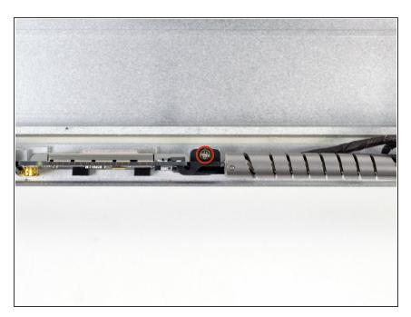
Remove the 2.7 mm Phillips #00 screw securing the AirPort board bracket to the rear display bezel.
