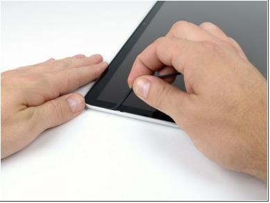
Starting with the freed corner, pull the left gasket off the left side of the display assembly.
