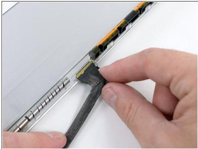
Carefully pull the display cable through its slot in the aluminum housing, rotating it as necessary to fit through the opening.
