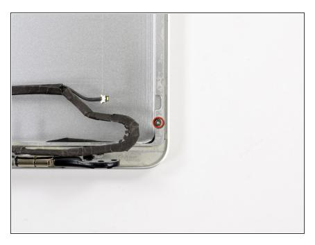
Remove the single 1.9 mm Phillips #00 camera cable screw.
