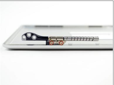
• Remove the three 5.2 mm T6 Torx screws securing the left clutch hinge to the rear display bezel.
