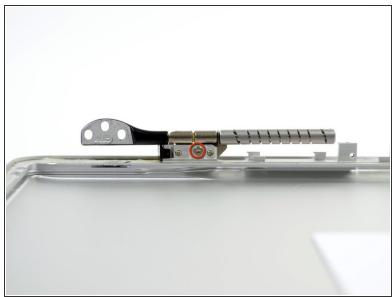
• Remove the three 5.2 mm T6 Torx screws securing the right clutch hinge to the rear display bezel.
