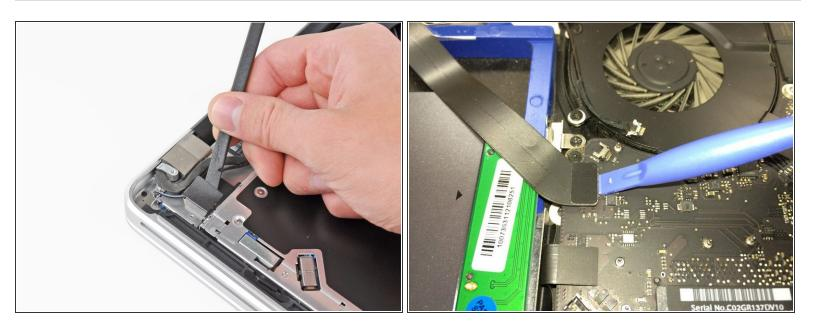
Use the flat end of a spudger to peel the thin plastic cover off the top and sides of the Bluetooth board housing. For late-2011 models check out the other picture because the connector location is in a totally different location.
