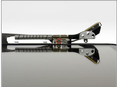
• Remove the three 5.2 mm T6 Torx screws securing the left clutch hinge to the display assembly.
