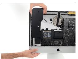
• Lift the left speaker straight up and remove it from the iMac.
