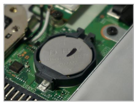
• Lift battery up and out with plastic spudger.
