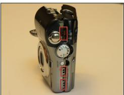
• Slowly pry apart the two covers from the bottom. When you have them apart about 1/4", take you finger and run it lightly along the top of the camera on the back cover side. This should release the three catches on the the shell.
