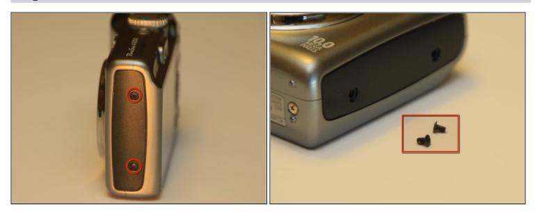
• On the right side of the camera, remove the two fine thread screws.
