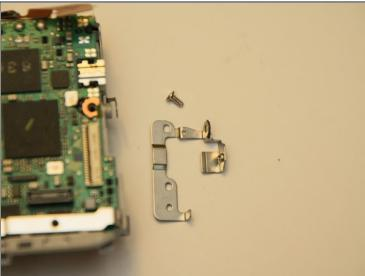
Remove the coarse thread screw from the upper keypad bracket.
