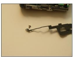
Remove the two fine thread screws on the top of the keypad. Then remove the one coarse thread screw holding the plastic piece in place on the side of the camera.
