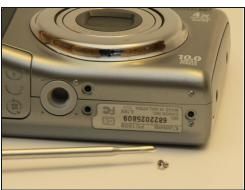
• Start by removing these three screws. The first two on the left are longer, coarse thread for the plastic, the one on the right is a fine thread that taps into the metal plate underneath.
