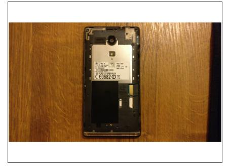
Remove 8 Phillips screws (one in center) and 2 smaller Phillips screws
