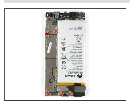
Remove the five Phillips #00 screws that hold down the motherboard of your Huawei P8.
