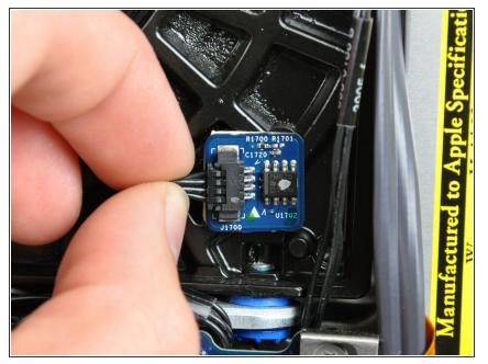
Disconnect the hard drive thermal sensor by pulling the connector away from its socket parallel to the face of the hard drive.
