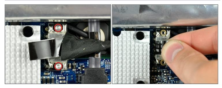
• Remove the two 5 mm T6 Torx screws securing the display data cable to the logic board.
