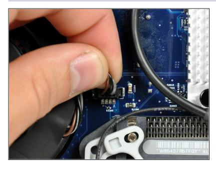
• Pull the CPU fan connector up off its socket on the logic board.
