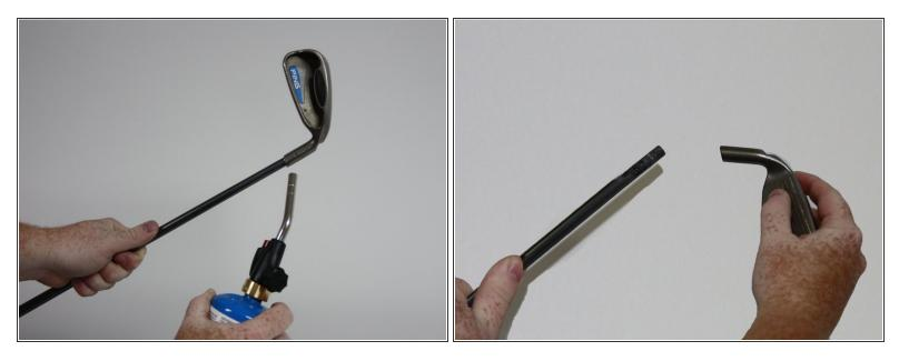
Using propane or a torch, heat the hosel of the club to remove the steel shaft from the club head.
