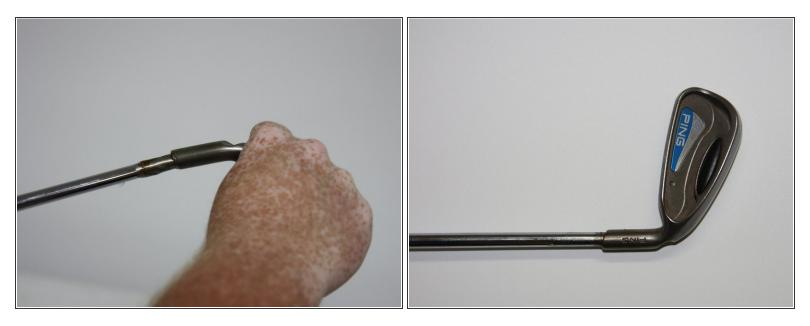
Insert the shaft into the club head. Hold the head and shaft together for approximately 30 seconds to secure.
