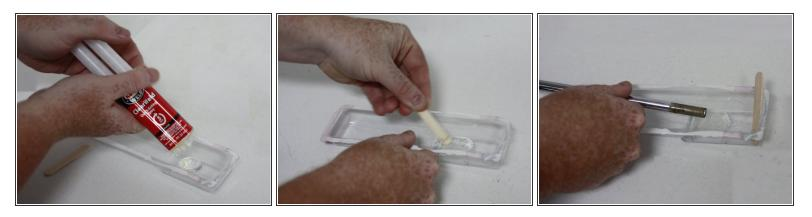
• Pour epoxy into a container and stir to mix it together. Once epoxy is mixed together, spin the shaft tip into the epoxy to prepare for insertion into the head.
