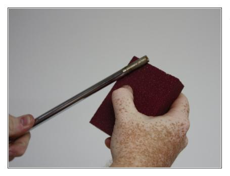
Use a piece of sand paper or a grinder to roughen the tip of the shaft where it connects to the hosel of the club head.
