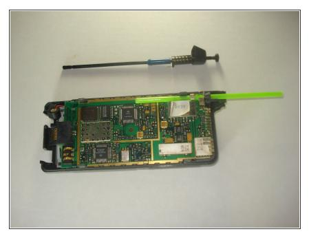
Slide the antenna out of the green tubing and slide the green tubing out of it's corresponding hole on the motherboard.
