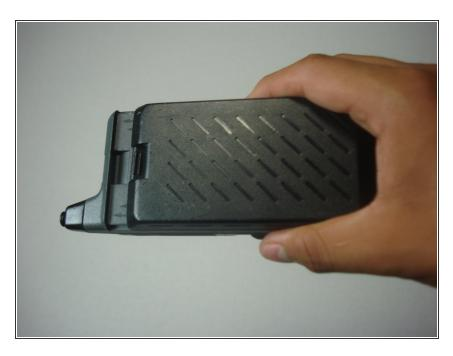
Remove the battery by sliding it down the rails to which it is connected.
