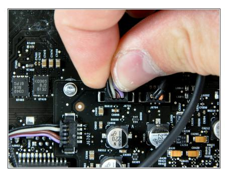
Disconnect the right speaker cable connector from the audio board by pulling it straight up from its socket.
