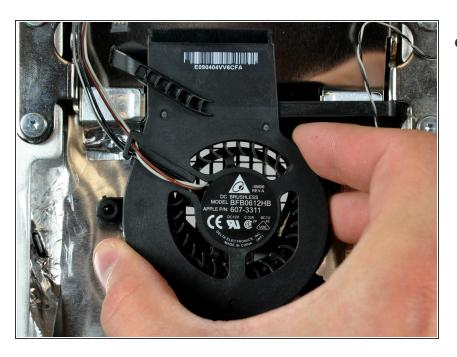
Gently lift the hard drive fan off the plastic pins protruding from the lower case.
