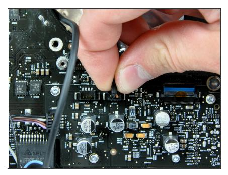
Disconnect the microphone cable connector from the audio board by pulling it straight up from its socket.
