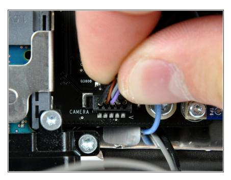
Disconnect the camera cable connector from the logic board by pulling it straight up from its socket.
