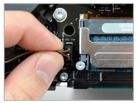
Disconnect the CPU fan connector from the logic board by pulling it straight up from its socket.
