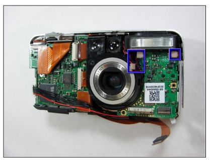
• Disconnect the two wired plugs below the flash.
