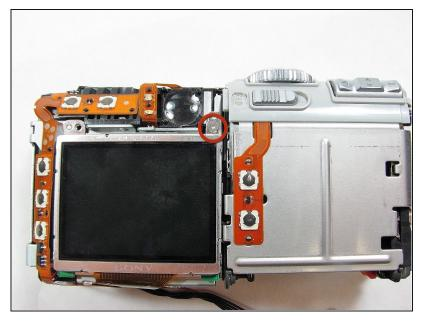
• Remove the 2.4mm screw located just to the upper right of the LCD Screen.
