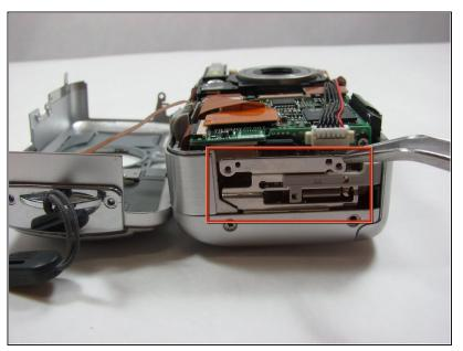
• Use a pair of <u>tweezers</u> and remove the metal piece inside the camera.
