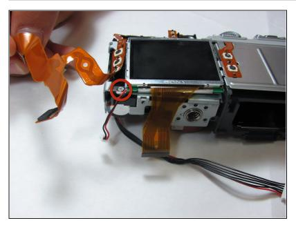
Remove the 3.3mm screw on the bottom left of the LCD screen.
