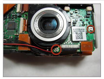
• Remove the two 3.4mm screws on the right motherboard.
