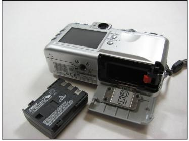
• Holding the edges, slide out the battery.
