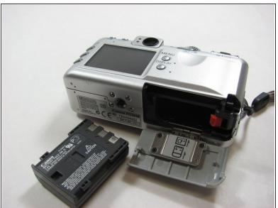
Holding the edges, slide out the battery.
