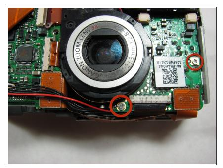
Remove the two 3.4mm screws on the right motherboard.
