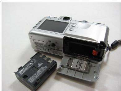
Holding the edges, slide out the battery.
